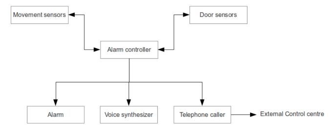
Which is intended to protect against intrusion and to detect fire. It incorporates smoke sensors, movement sensors, door sensors, video sensors, video cameras under computer control, located at various places in the building, an operator console where the system status is reported, and external communication facilities to call the appropriate services such as the police and fire departments. Draw the block diagram of a possible design for such a system.
