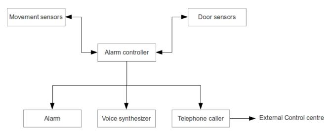
Which is intended to protect against intrusion and to detect fire. It incorporates smoke sensors, movement sensors, door sensors, video sensors, video cameras under computer control, located at various places in the building, an operator console where the system status is reported, and external communication facilities to call the appropriate services such as the police and fire departments. Draw the block diagram of a possible design for such a system.
